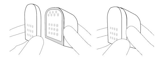
After using a mouthpiece, remove it from the sensor and wash it thoroughly with warm water and soap or wash it in a dishwasher. To sterilize the mouthpiece, you can use a food-grade alcohol wipe.
