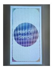
While the sensor is doing the preliminary measurement DON'T put the sensor on the meat.
