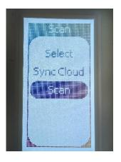
Turn on the sensor, go into the Scan menu, and choose either a batch number in Select or Scan.
