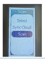
Turn on the sensor, go into the Scan-menu and choose either a batch in **Select** or a basic **Scan**.
